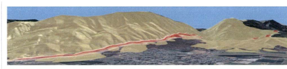
Figure 2: Computer image of the Santaquin east bench (looking southward up Santaquin Canyon), illustrating debris flow (yellow) and fault zone (red) hazards.
