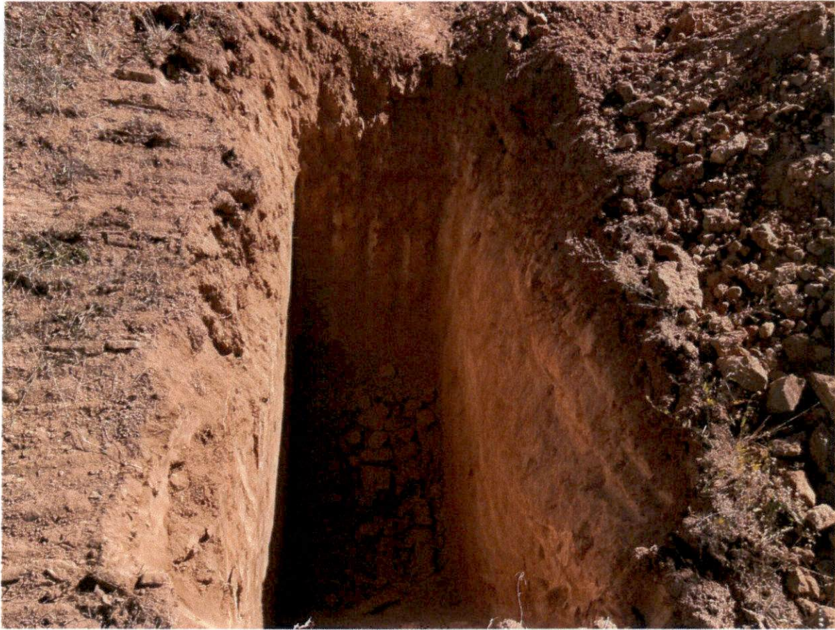
Hole 1 on Pipeline Centerline. Uniform sandy silt to 10 feet deep (pipeline invert)
